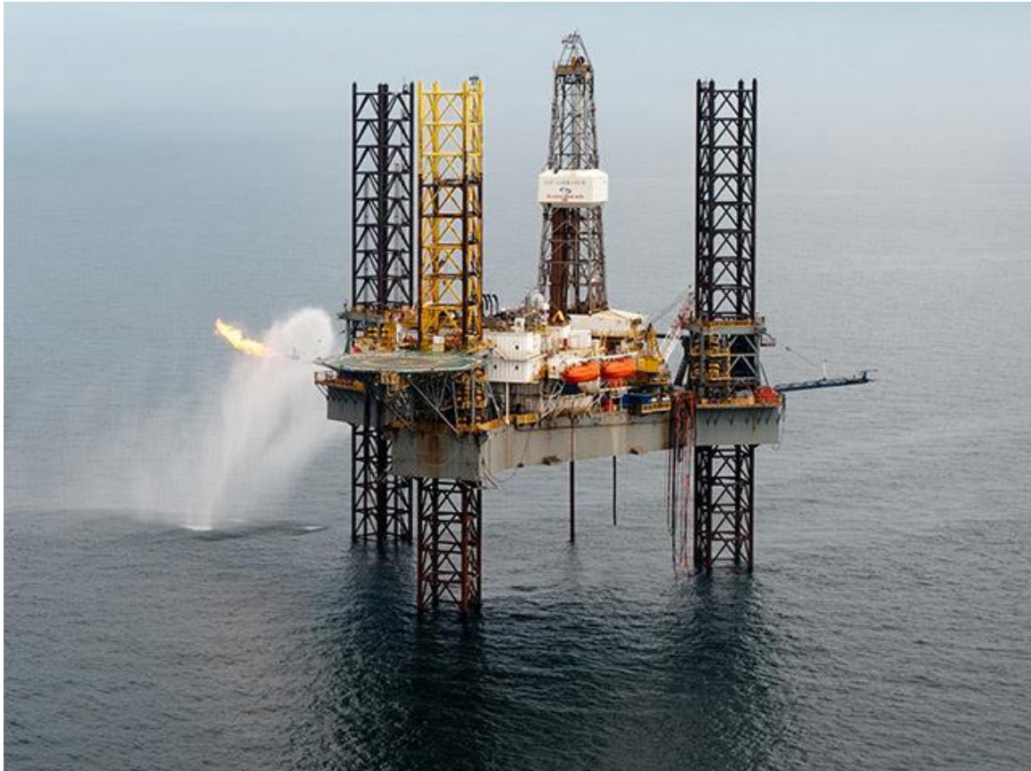
GSF Labrador jack-up drilling rig at the Platypus prospect in the North Sea for Parkmead and Dana Petroleum.
